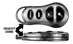
**Separating Transmitter Halves**
